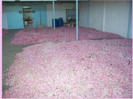
The fresh petals from that day are laid out to dry for 24 hours for solvent extraction of the absolute (2 floors high)
